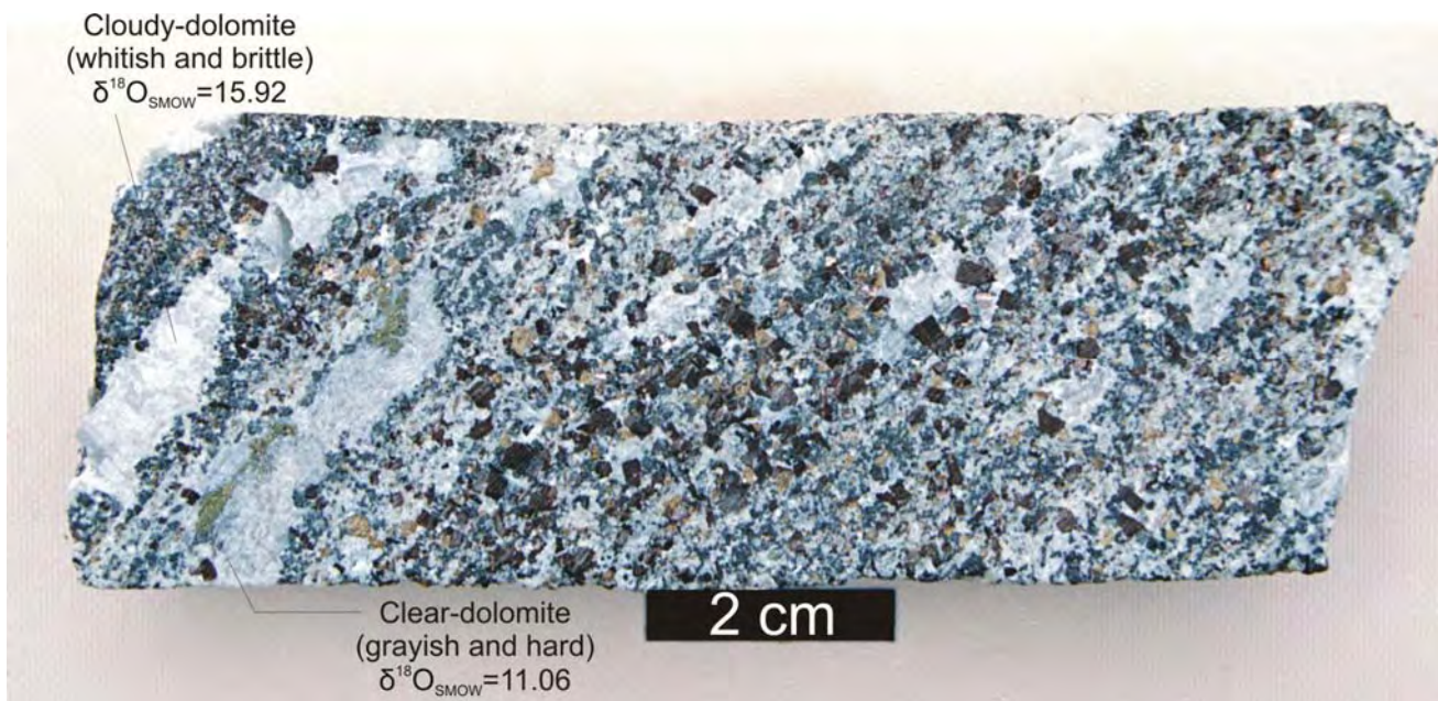
Fig. 4.12 Comparison between the hand-sample aspect of cloudy and clear carbonates in P2 (sample 178). Cloudy dolomite is more white and brittle compared to clear dolomite, and represents the recrystallisation product of primary (high-SrO) carbonates.
