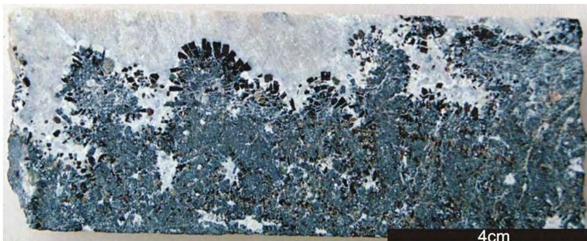
Fig. 4.5 P3 nelsonite with dolomite carbonatite pockets. Note the growth of tetra-ferriphlogopite in the boundary between P3 and the DC pocket, where ilmenite and apatite are also common.
