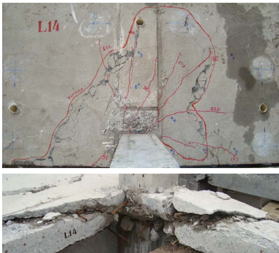
Figura 4.138 – Ruptura da laje do Modelo L14 – P_{1D}/P_{1E} = 2,0 ; P_2 = 40,0 MPa.
