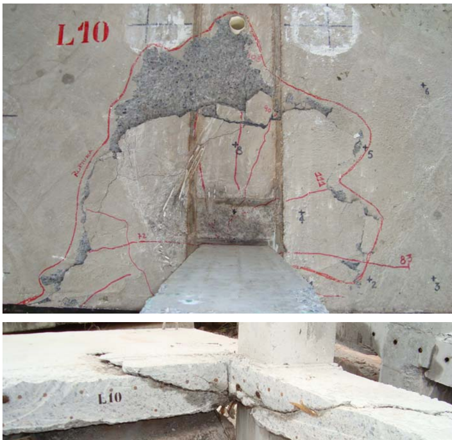
Figura 4.134 – Ruptura da laje do Modelo L10 – P_{1D}/P_{1E} = 4,0 ; P_2 = 40,0 MPa.
