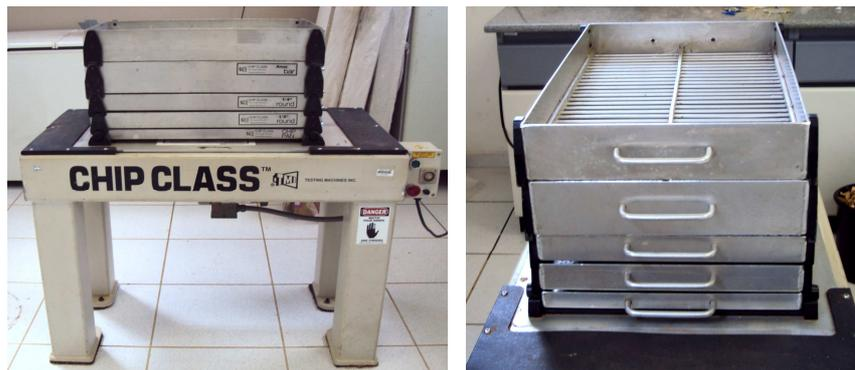
Figura 3 - Conjunto de peneiras Chip Class TMI - Testing machines Inc.
