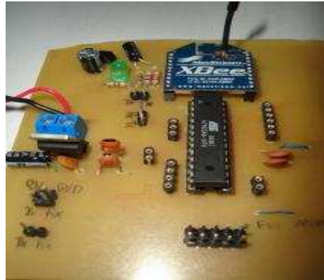
Figure 5. Diagram of the End Device Actuator (Filho and Dias, 2008).
