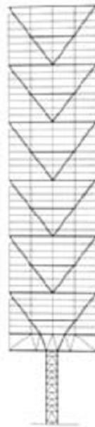
Figura 2.14 – Corte vertical do Citicorp Building (www.nyc-architecture.com)
