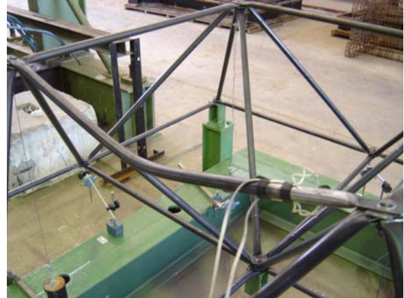
Figura 9.3 – Colapso global ( P=36\text{kN} )
