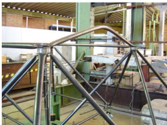
Figura 9.4 – Colapso global ( P=42\text{kN} )
