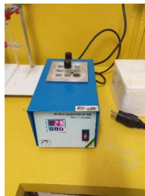
Bloco digestor (DQO)
