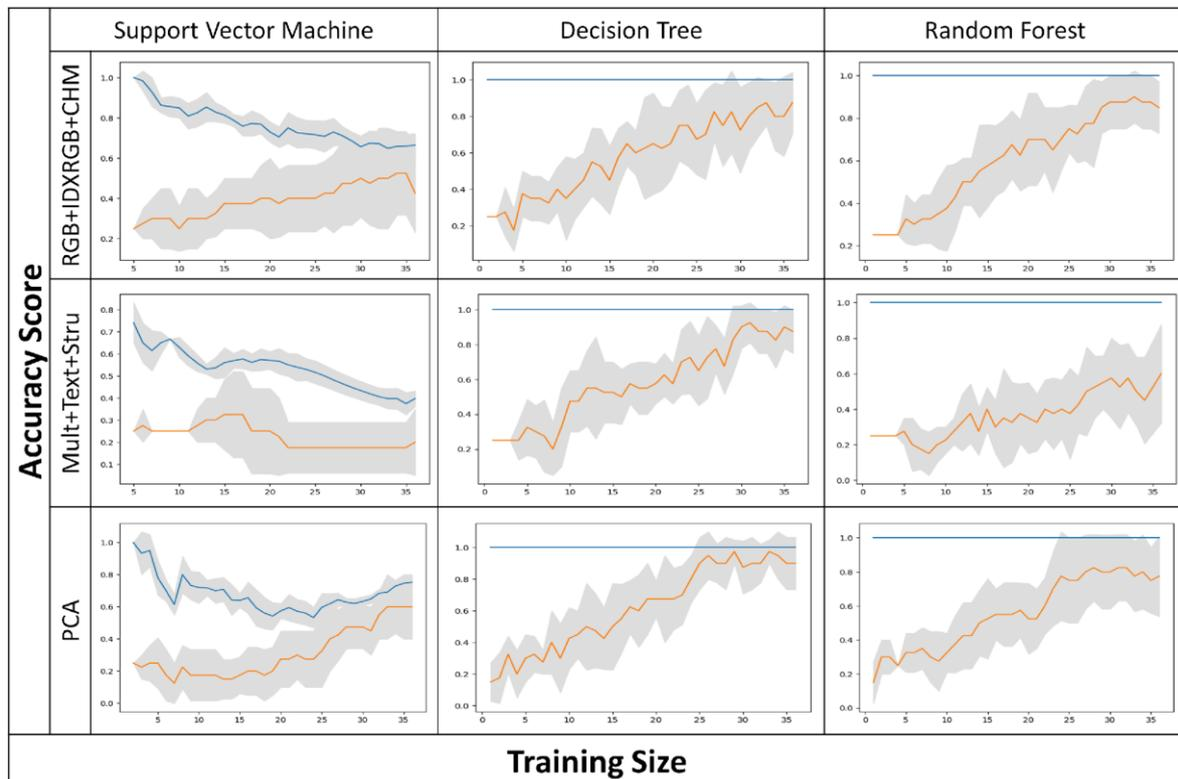
**Figure 5.** Learning curves relating to classification models: Support Vector Machine (SVM), Decision Tree (DT) and Random Forest (RF) and input layers from subset for *in situ* validation of wet season orthomosaic. The blue and orange lines with their standard deviation (SD) are the training and cross-validation mean scores, respectively. For abbreviation identification of input layers, see Table 1.
