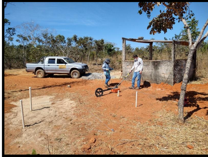
Figure 4 - Photograph of the GPR data acquisition in the controlled site area with the 400 MHz antenna.
