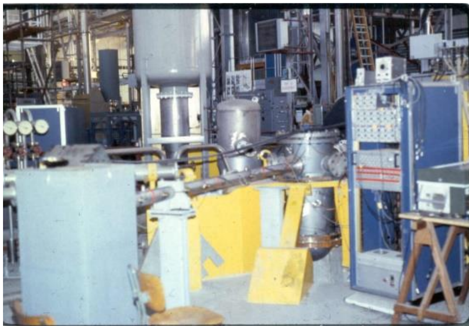
Figure 2-20 - SAFRAN circuit, representing a simplified scale model of a PWR reactor
