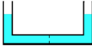
Figure 1-4 - A simple scheme of the TLCD
