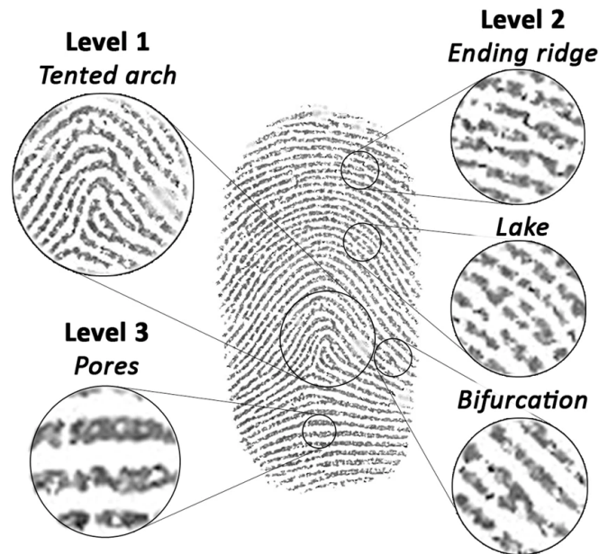
Figure 3.2: The 3 levels of analysis of a fingerprint. Image replicated from Scotcher and Bradshaw (2018).
