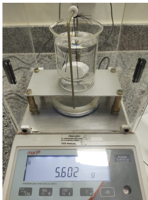
Figure 3.7 – The set-up used to measure immerse mass of a sample.
