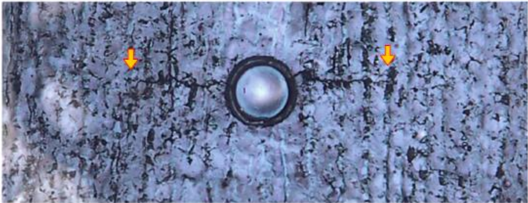
Figure 1.2 - Crack with a length of 392 \mu\text{m} formed at a hole with a diameter and depth of 100 \mu\text{m} (modified from [7]).
