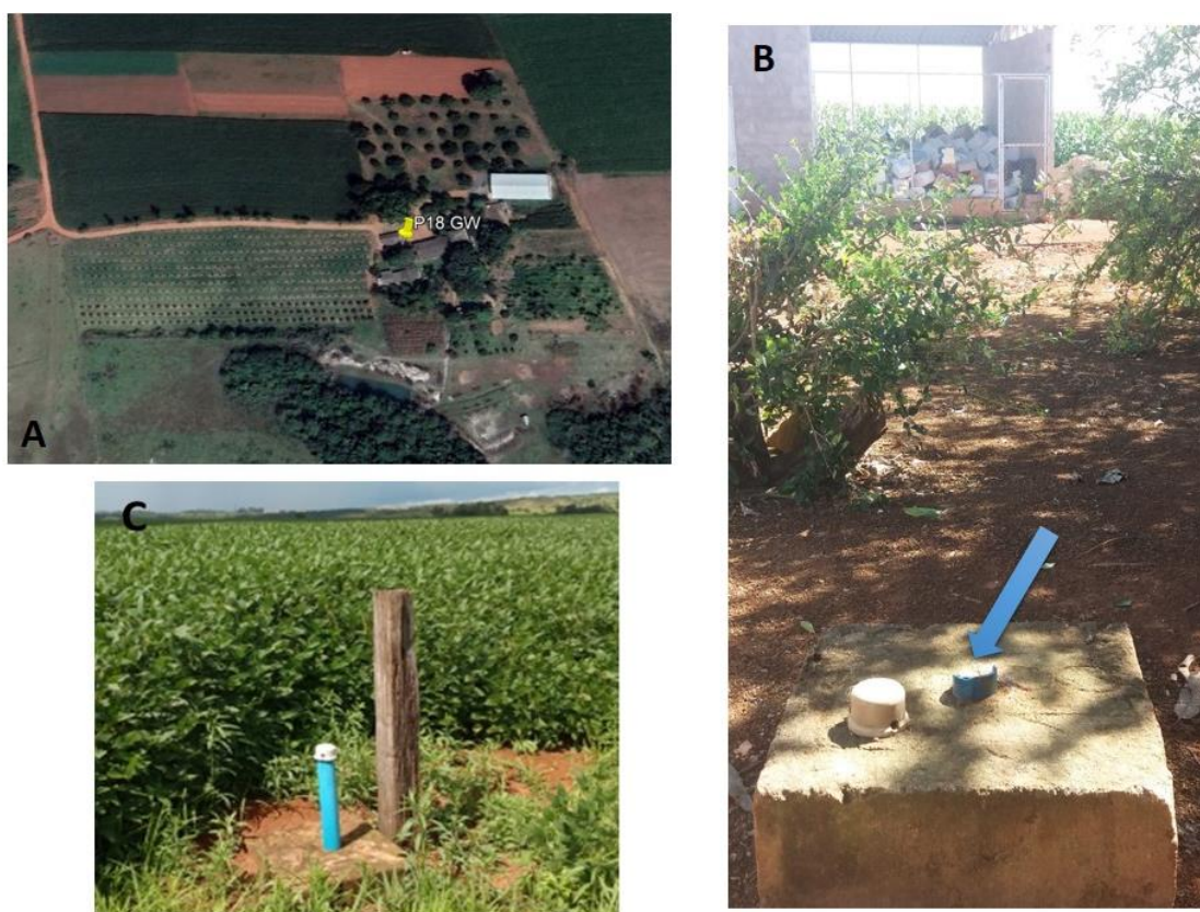
Figure S1 A: Aerial view (source: Google Earth) of P18GW sampling point area in the Rio Preto Hydrographic Basin. B: detail of the P18GW sampling point (piezometric well, blue arrow), showing the empty pesticide packing storage room in the background; C: P24 sampling point in the middle of a soybean field .
