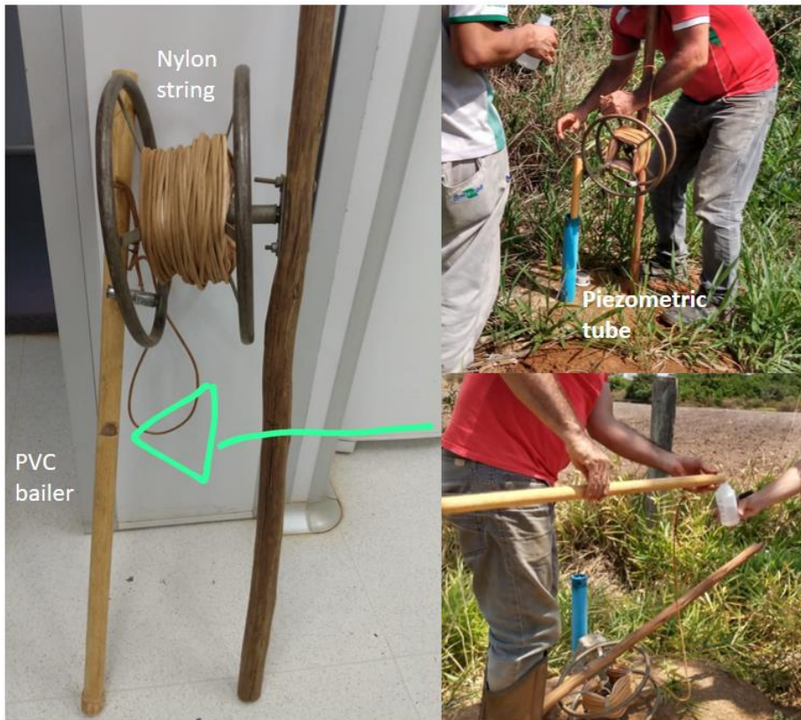
Figure S2 Groundwater sample collection in the piezometric well in the Rio Preto Hydrographic Basin. The green arrow shows the opening in the bailer for water collection
