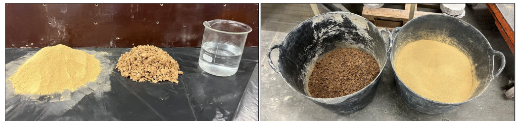
Figure 14. Proportions of soil, dispersed fibres, and water in Kraftterra.
