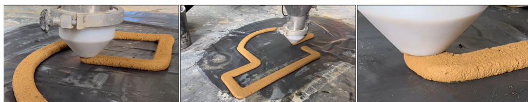
Figure 16. Smooth Finish Printing. An RPSEF was used that produced extrusion strands with the same width as the extrusion nozzle's exit diameter.
