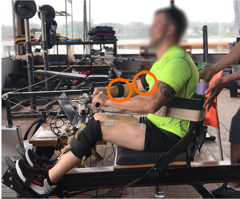
Figure 5.11: SCI participant in the final FES-rowing experimental setup. Both IMUs are highlighted in orange.
