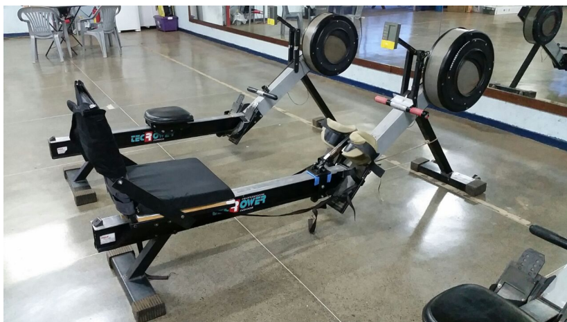
Figure 5.10: Comparison between the adapted rowing machine and a standard one. Note the seat for trunk stabilization, the custom device for legs stabilization, and the safety straps.
