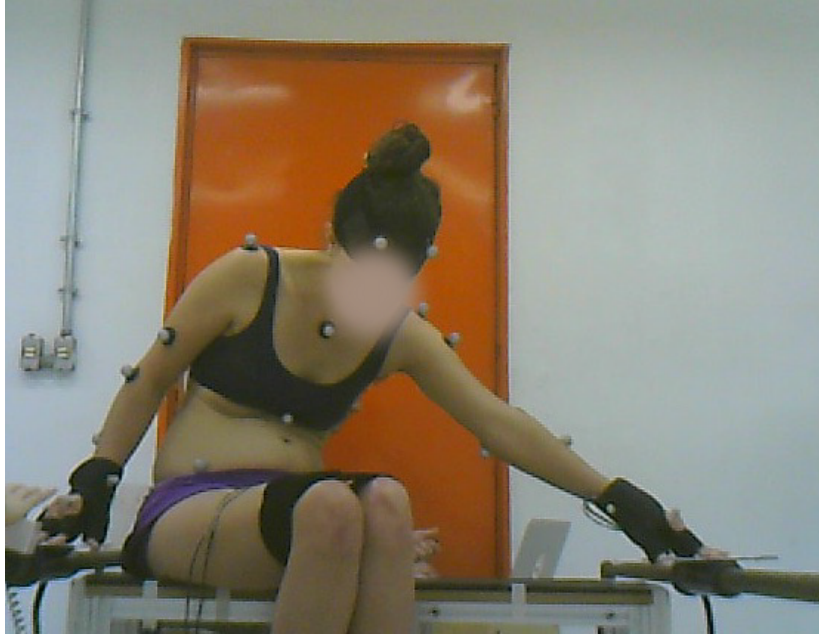
Figure 4.3: Transfer experimental set-up. The gloves embed pressure sensors. It is possible to see the markers over the subject body, whose 3D positions are captured by the motion capture system. The benches are next to each other, with a 10^\circ angle between them. The legs are constrained to keep them for falling sideways.
