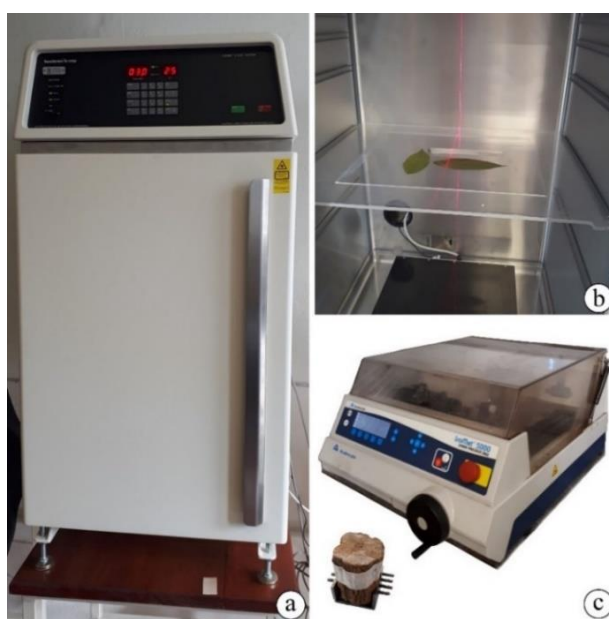
Figure 3. Equipment used for X-ray techniques. a-b. Faxitron MX-20 digital radiography system; c. IsoMet 5000 linear precision saw and wood sample.
