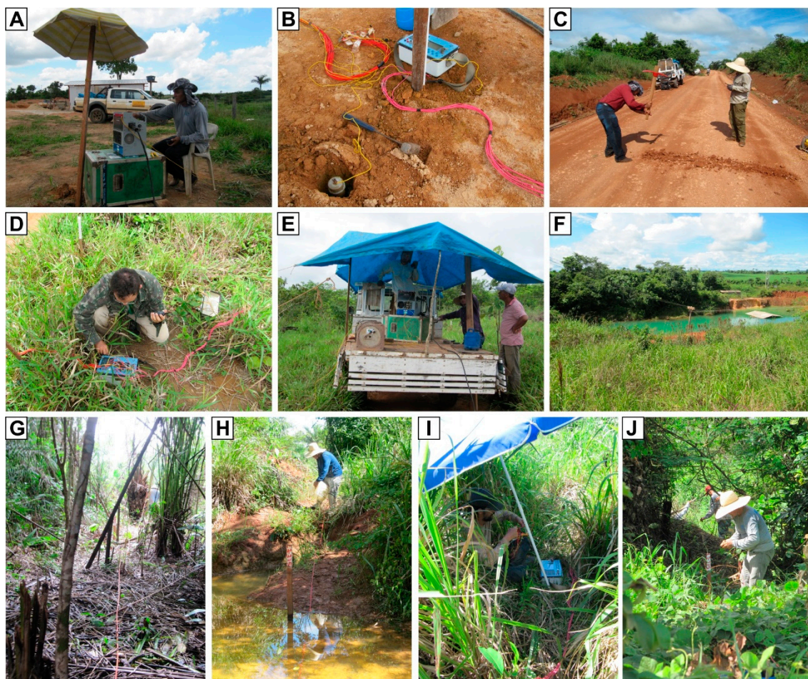
Figure 8. Photos showing some geoelectric data acquisition stages in the surveyed mines: (A) electric transmitter in operation; (B) data receiver and porous electrode used for recording electrical potential; (C) excavated trench for protection of electrical cables; (D) receiver operation in the field area; (E) tent mounted on a truck for protection of electric transmitter; (F) caves bypassed during the measurements; (G) open pathway in palm forest; (H) aerial transposition of electrical cables over a body of water; (I) open pathway in pasture area; and (J) mounting electrodes in a closed forest area.
