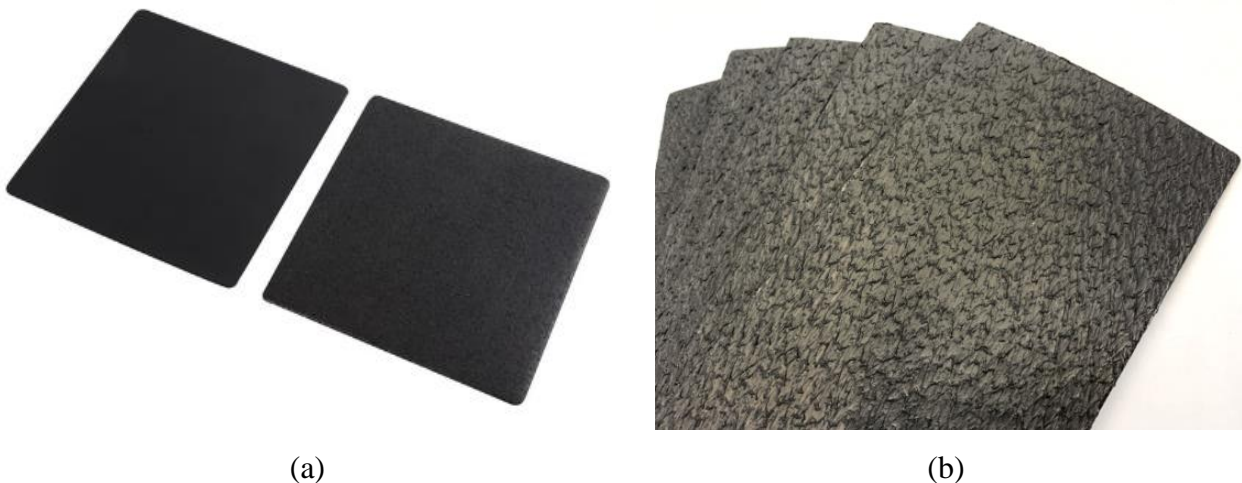
Figure 2.3. HDPE geomembranes: (a) Smooth, and (b) Textured (Cen et al. 2018).
