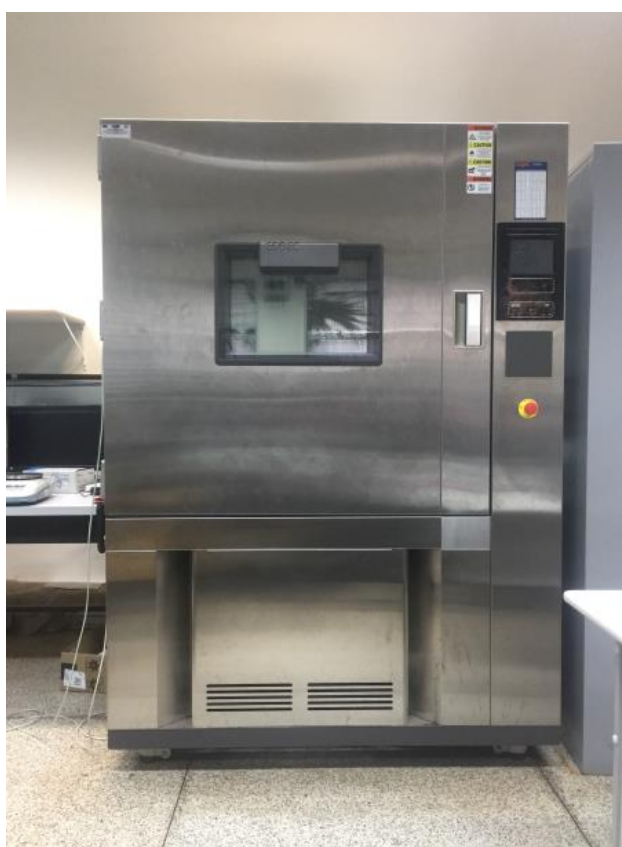
Figure 6: Platinous EPL-4H Climatic Chamber. Source: From Barella [2021].
