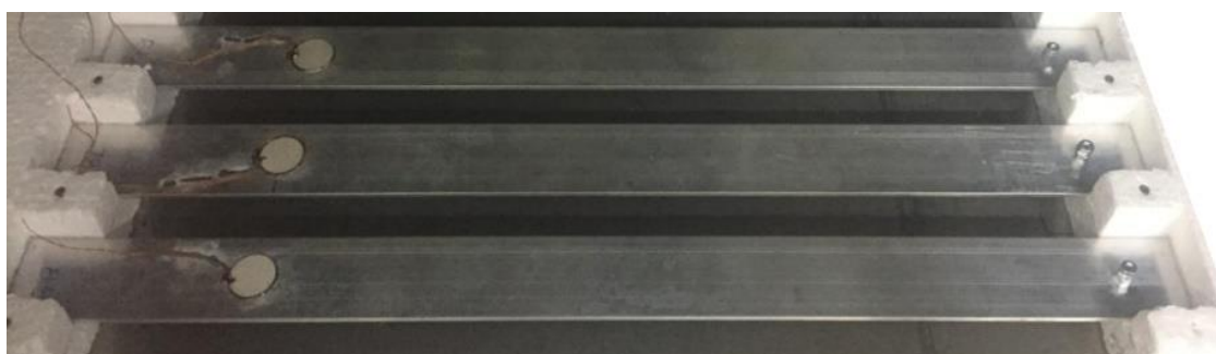
a) Structural Systems (Aluminum Beams + PZTs Insert).
