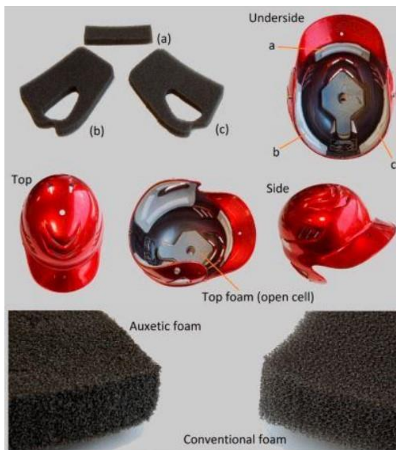
Figure 12: Foam inserts: (a) foreheads, (b) right side and (c) left side [Shepherd et al., 2020].
