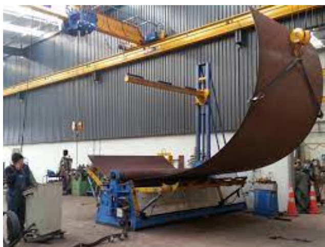
Figure 13: Bend plates for oil tanker ships [22]
