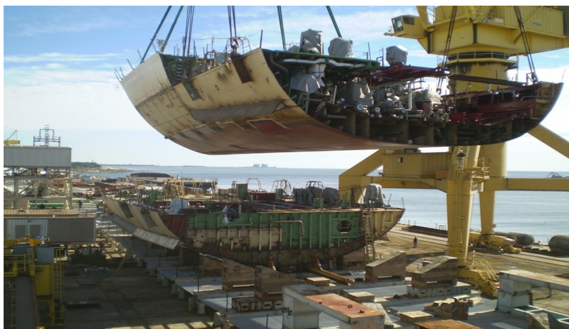
Figure 8: Ship modular construction in a shipyard [15]
