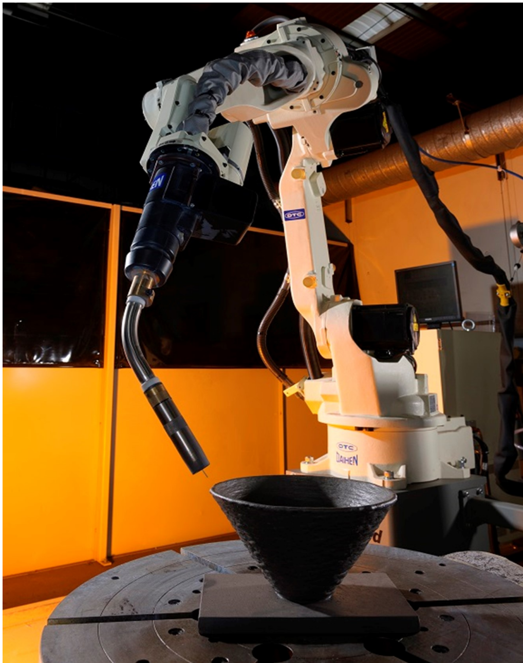
Figure 14: WAAM system used at TMI (Office) [2022])
