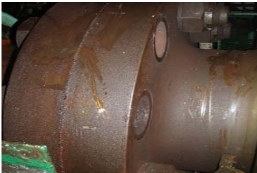
Figure 16: example of fretting in a ship shaft [25]
