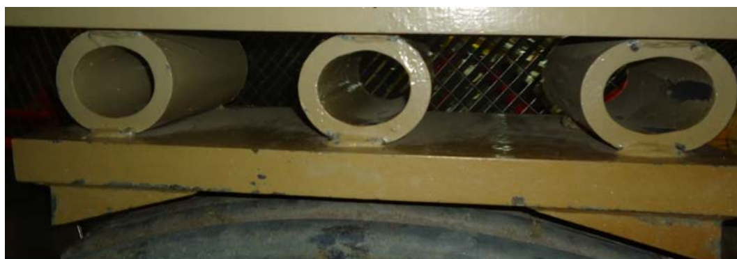
Figure 17: deformed pipe whip Restraints (top view)
