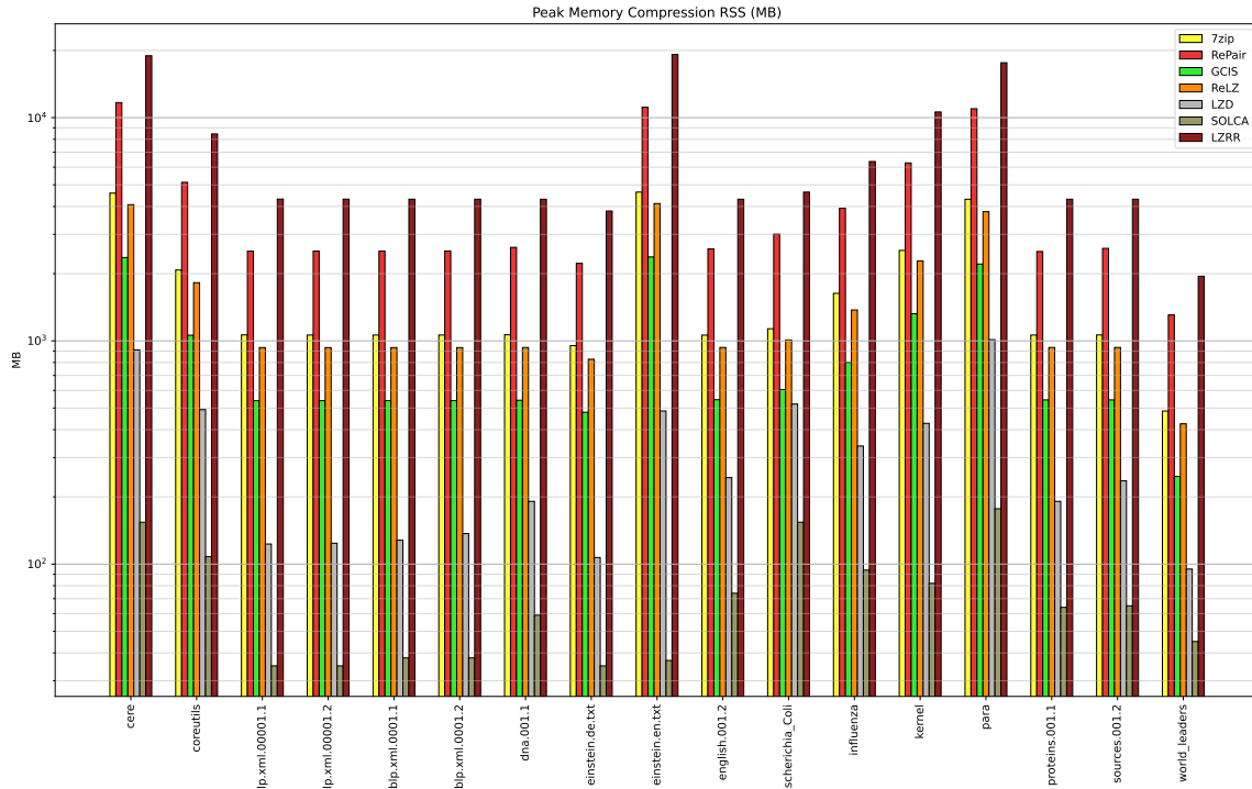
Figure 5.11: Peak memory (in MB) used by the compressors during compression for repetitive texts.
