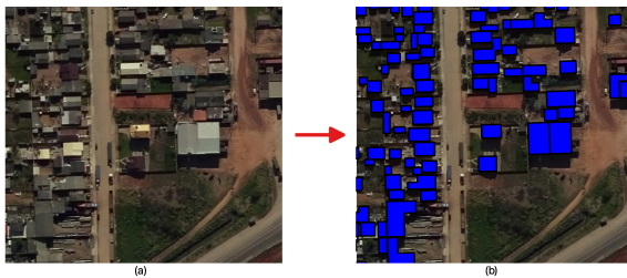
Fig. 2: Example of image (a) and extracted building footprint overlaid on the image (b)
