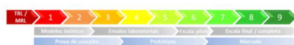
Figura 21: Adaptado de Níveis de maturidade tecnológica: Escala TRL/MRL baseada na referência primária ISO/FDIS 16290:2013 (E) Space systems – Definition of the Technology Readiness Levels (TRLs) and their criteria of assessment. International Organization for Standardization, Switzerland, 2013, 12 p.
