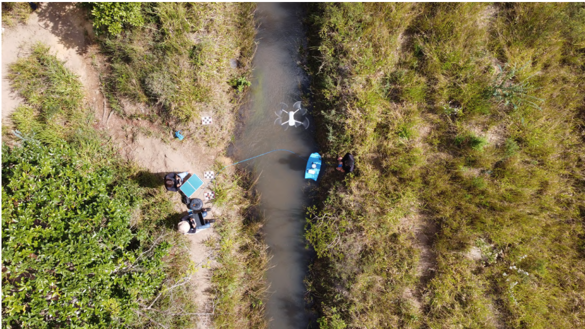
Figure 2.1 – Field setup with the ADCP and the Drone at the Rodeador Channel
