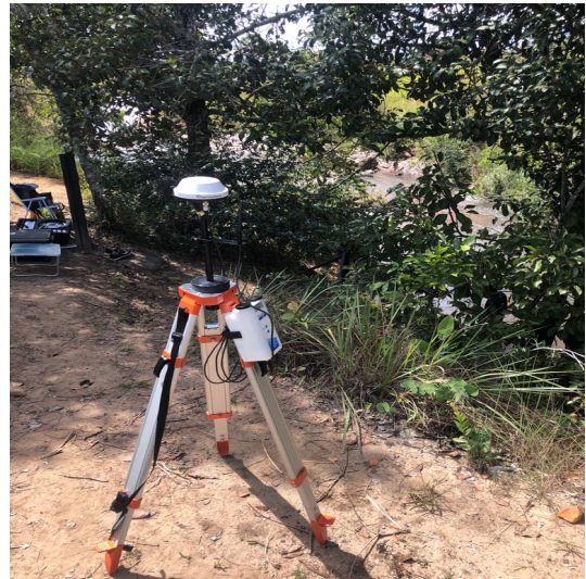
(b) RTK Base Station
