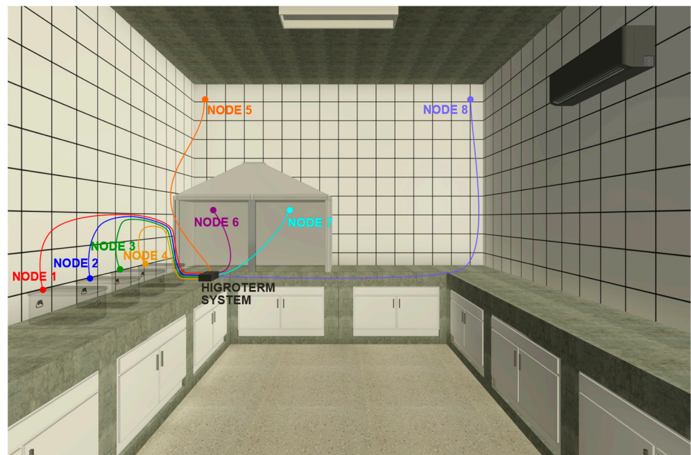
Figure 11. Example of test setup for material testing with the use of the HIGROTERM system.
