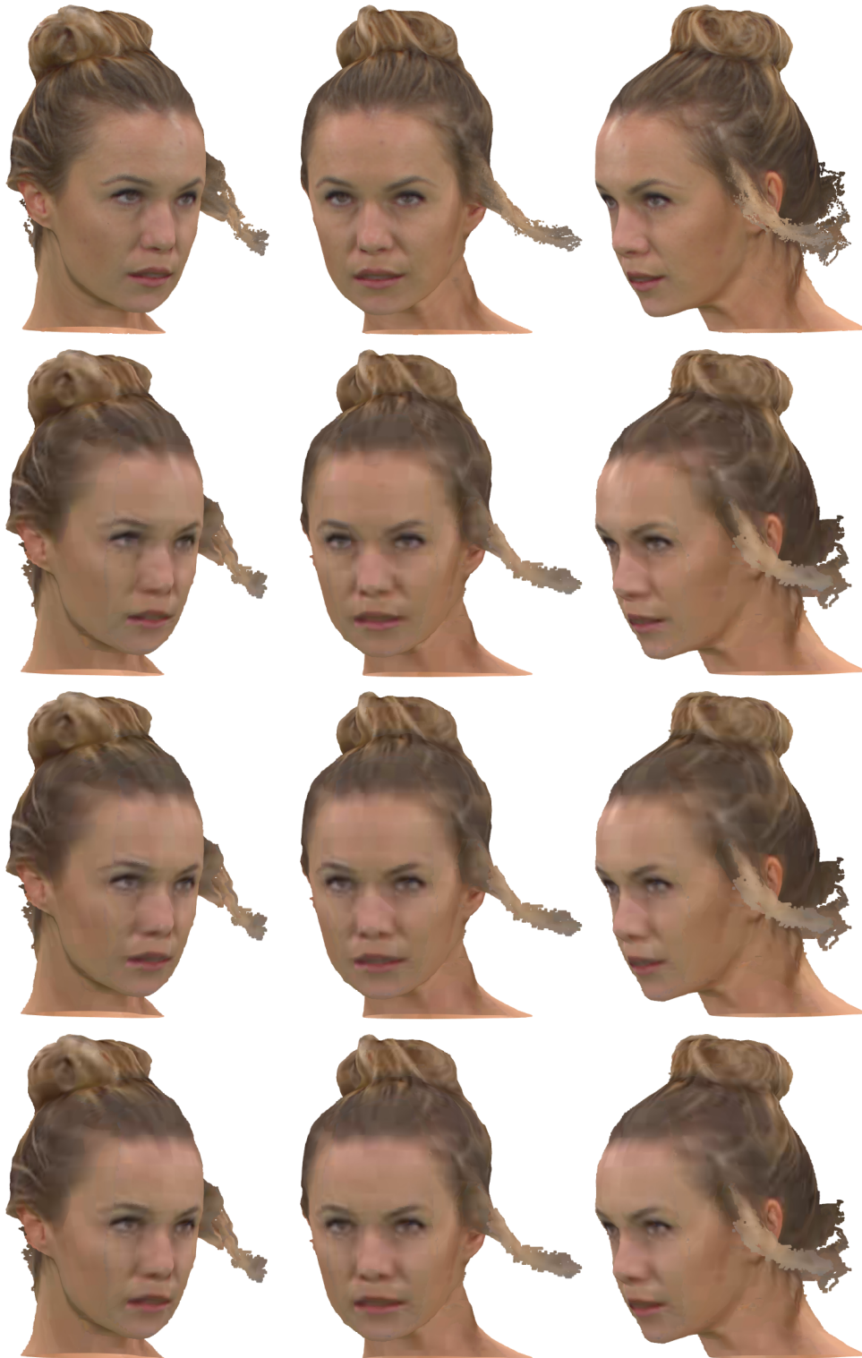
Figure 5.15: Decoded views (cameras 1, 2 and 3) of the plenoptic Longdress PC. From top to bottom: original point cloud; conventional V-PCC, where the plenoptic data occupies 8488000 bits, or 9193136 bits when considering the default RGB value triplet, in both cases with a PSNR of 34.5 dB with respect to the original point cloud; plenoptic differential coding, where the plenoptic data occupies 968080 bits when considering RGB, with a PSNR of 34.3 dB; plenoptic non-differential coding, where the plenoptic data occupies 876160 bits, with a PSNR of 34.1 dB.
