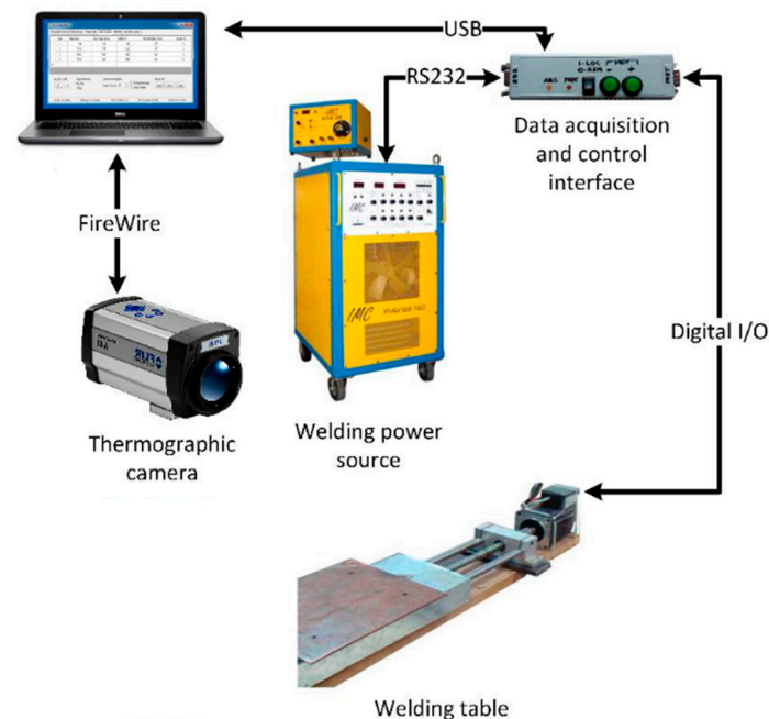
Figure 2. Schematic overview of components and connections of data acquisition and open-loop control system. Adapted from [13].
