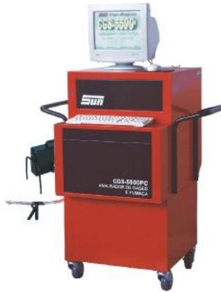
Figura 3.6 – Analisador de Gases e Fumaça Sun CGS-5500 PC (Snaponsun, 2008)
