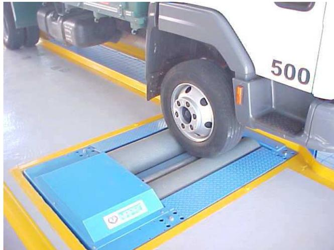
Figura 3.12 – Frenômetro – DNI/CT/UNICAMP (Novaes, 2006)
