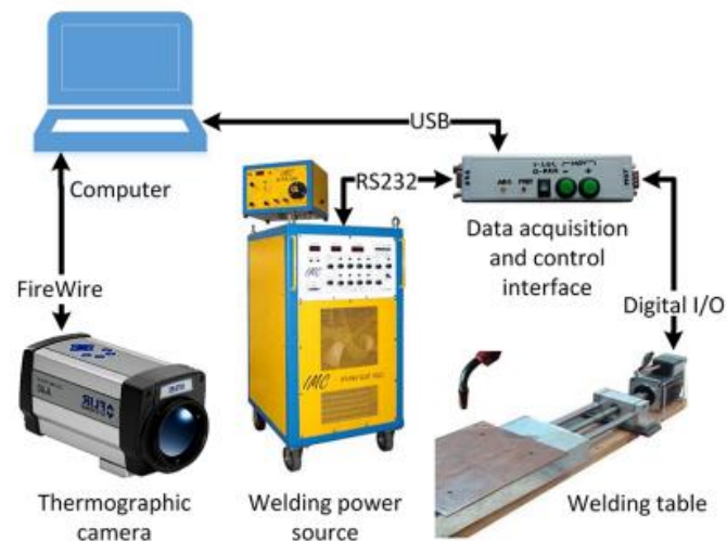
Figure 4.2 - Schematic overview of components and connections of data acquisition and open loop control system (BESTARD; SAMPAIO; ALFARO, 2018).
