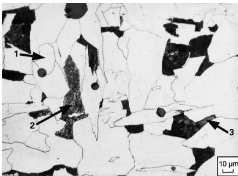
Figure 3.25 - Intragranular primary ferrite and pearlite in as cast, 0.13%C, 2.0%Mn, cerium sulfide particle dispersed steel where (1) indicates idiomorphic ferrite, (2) indicates ferrite - carbide aggregate and 3 indicates irresolvable pearlite Thewlis (2004).
