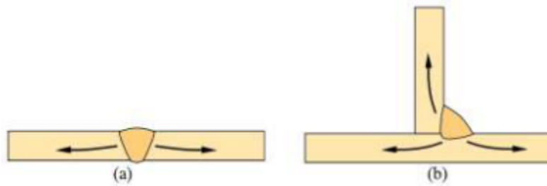
Figure 3.44 - Heat dissipation when welding (a) top and (b) "T" joints (MODENESI; MARQUES; SANTOS, 2012).
