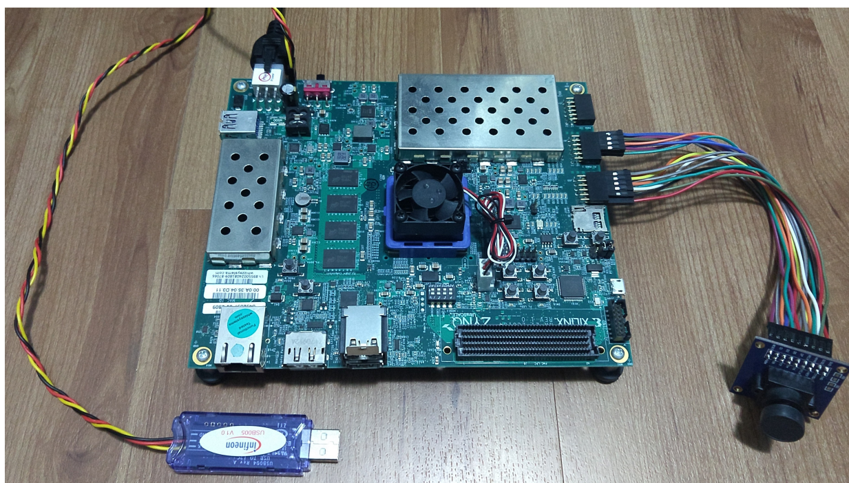
Figure 6.9: Photography of the ZCU104 Development Kit with the OV7670 CMOS sensor and the Infineon power monitor device.
