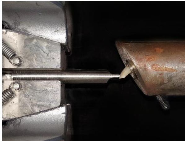
Figure 32 The specimens mounted in a universal testing machine.
