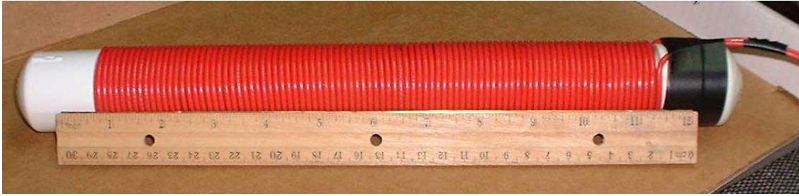
Figure 3.8: Ferrite rod antenna Source: Souterweb [55]
