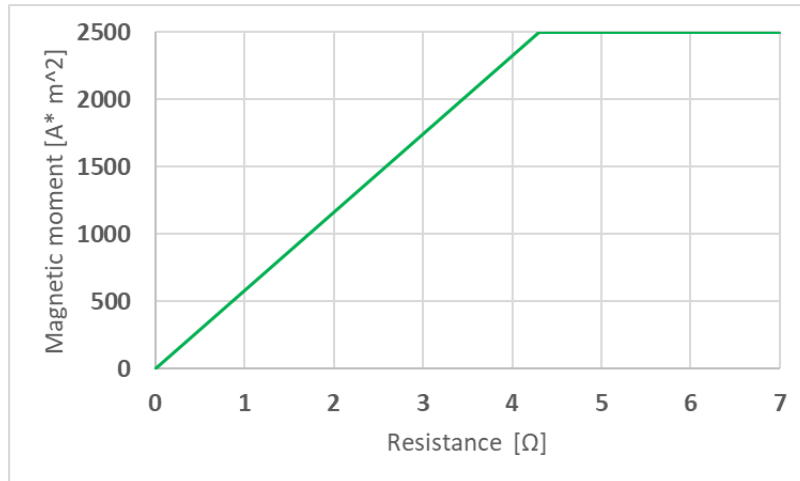
Figure 5.15: Relationship between the resistance and the magnetic moment of the antenna to obtain the maximum voltage-current ratio from the power amplifier.
