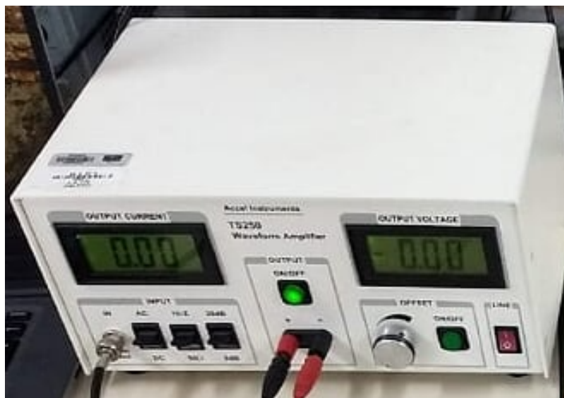
Figure 5.2: Power amplifier used for transmission on some tests.
