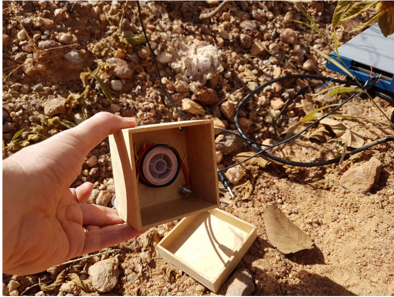
Figure 5.10: Tag antenna # 0 for TTE communication with 11 g of AWG 32 copper and transverse area of 1,76 \times 10^{-6} \text{ m}^2 .
