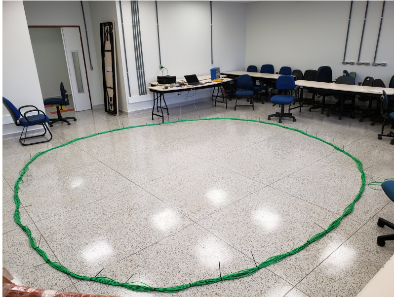
Figure 5.13: Flexible wire antenna for TTE communication with a 6 \text{ mm}^2 cross-section 240 \text{ m} copper flexible wire with transverse area of 19.63 \text{ m}^2
