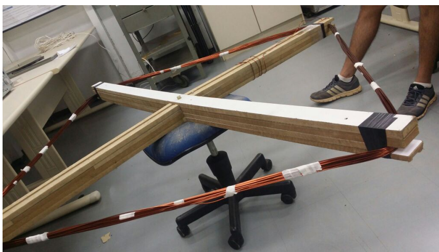
Figure 5.7: Square antenna for TTE communication with 4.9 Kg of AWG 11 copper and transverse area of 1.72 m 2 .
