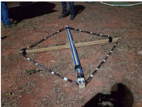
(a) Square antenna # 1 used for up-link reception.
