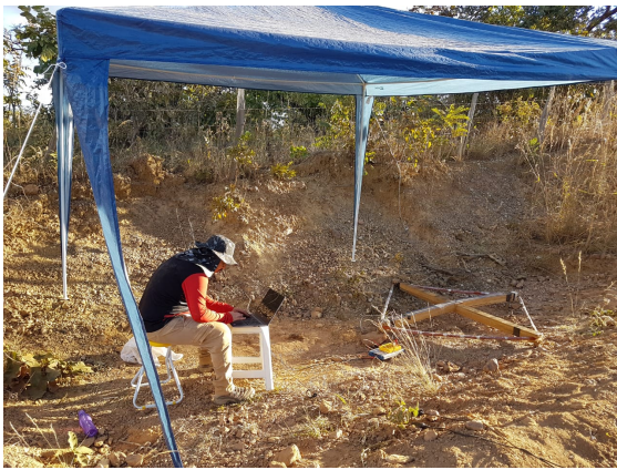
(a) Square antenna # 1 used for up-link reception.
