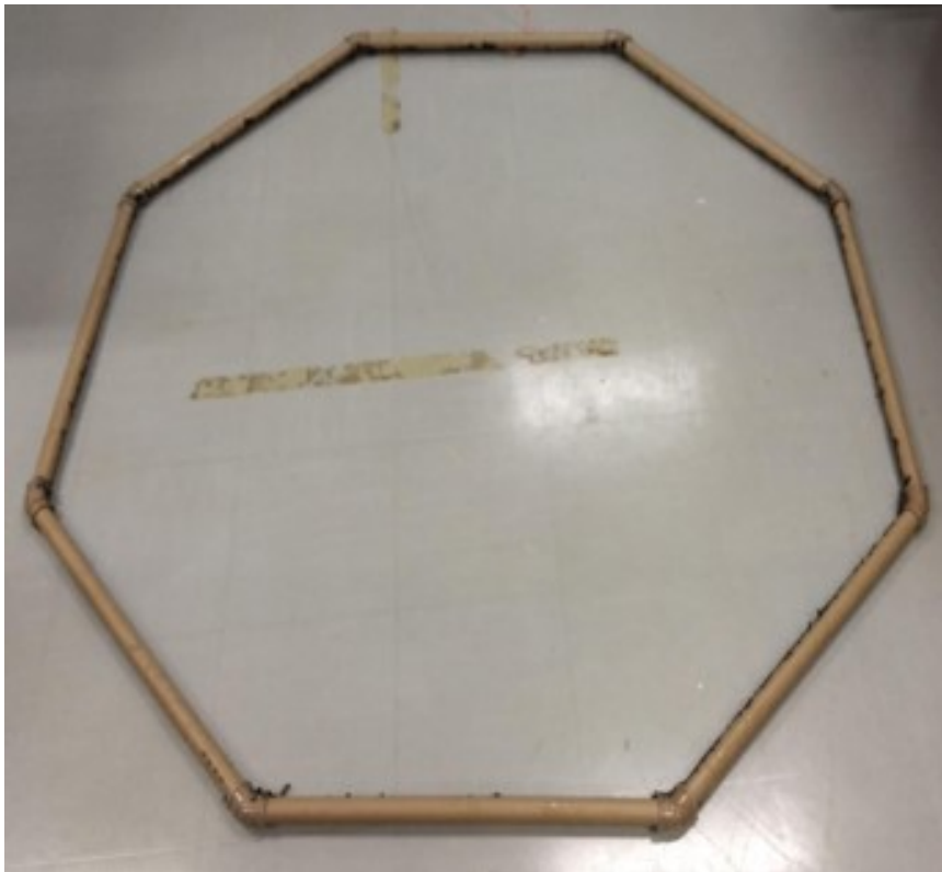
Figure 5.8: Octagonal antenna for TTE communication with 2.79 Kg of AWG 11 copper and transverse area of 2.43 m 2 .
