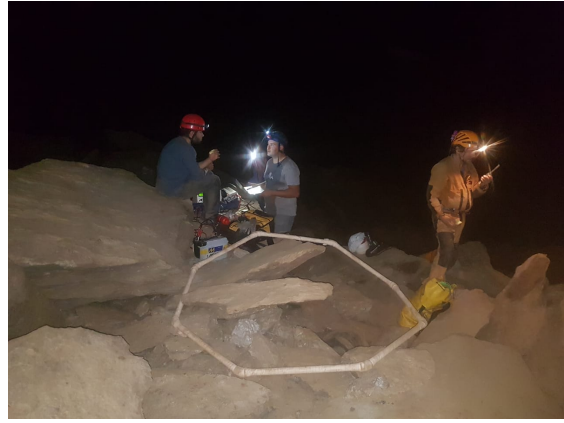
(b) Octagonal antenna used for up-link transmission.
