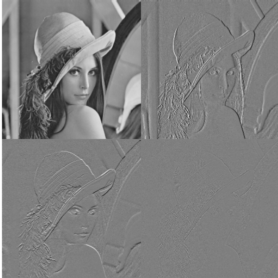
(c) Transformed coefficients after applying Haar transform over the columns and then horizontal axis
