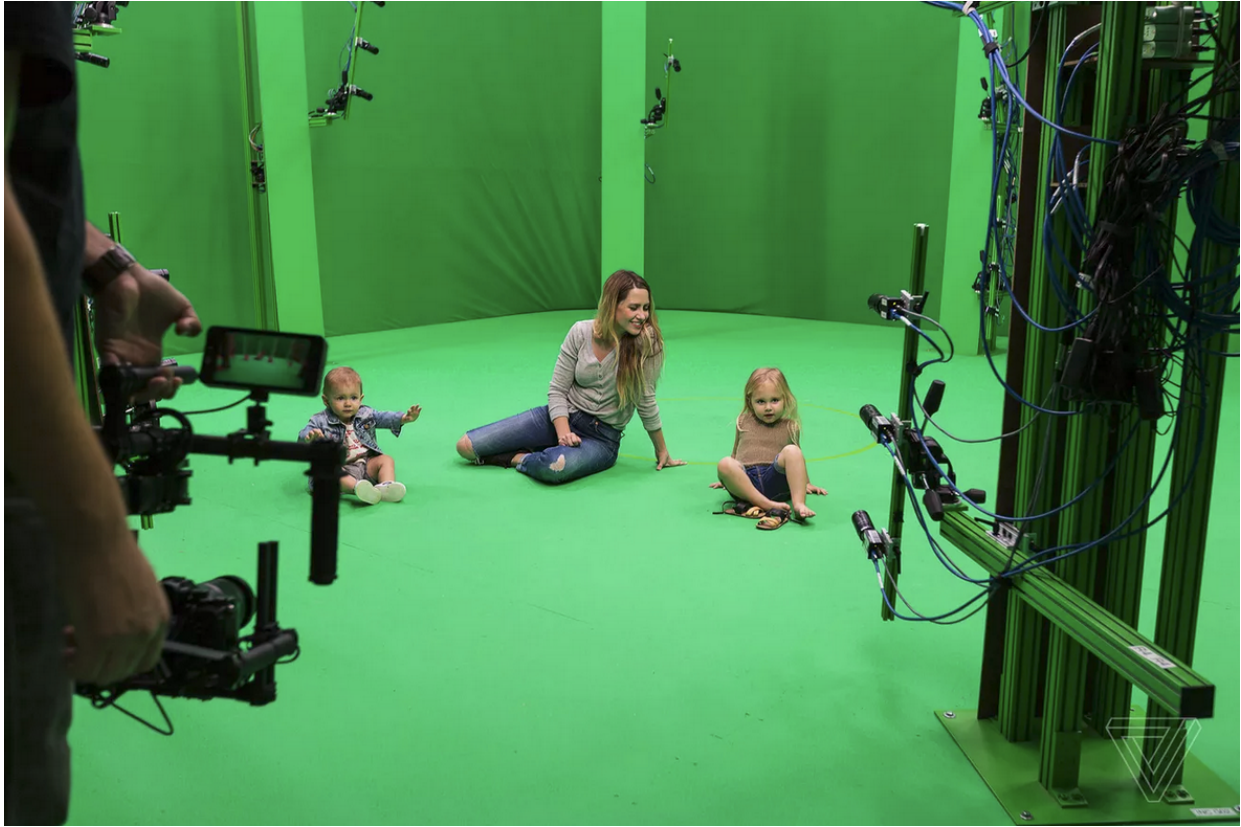
Figure 2.3: Array of cameras capturing a point cloud at 8i [20].
