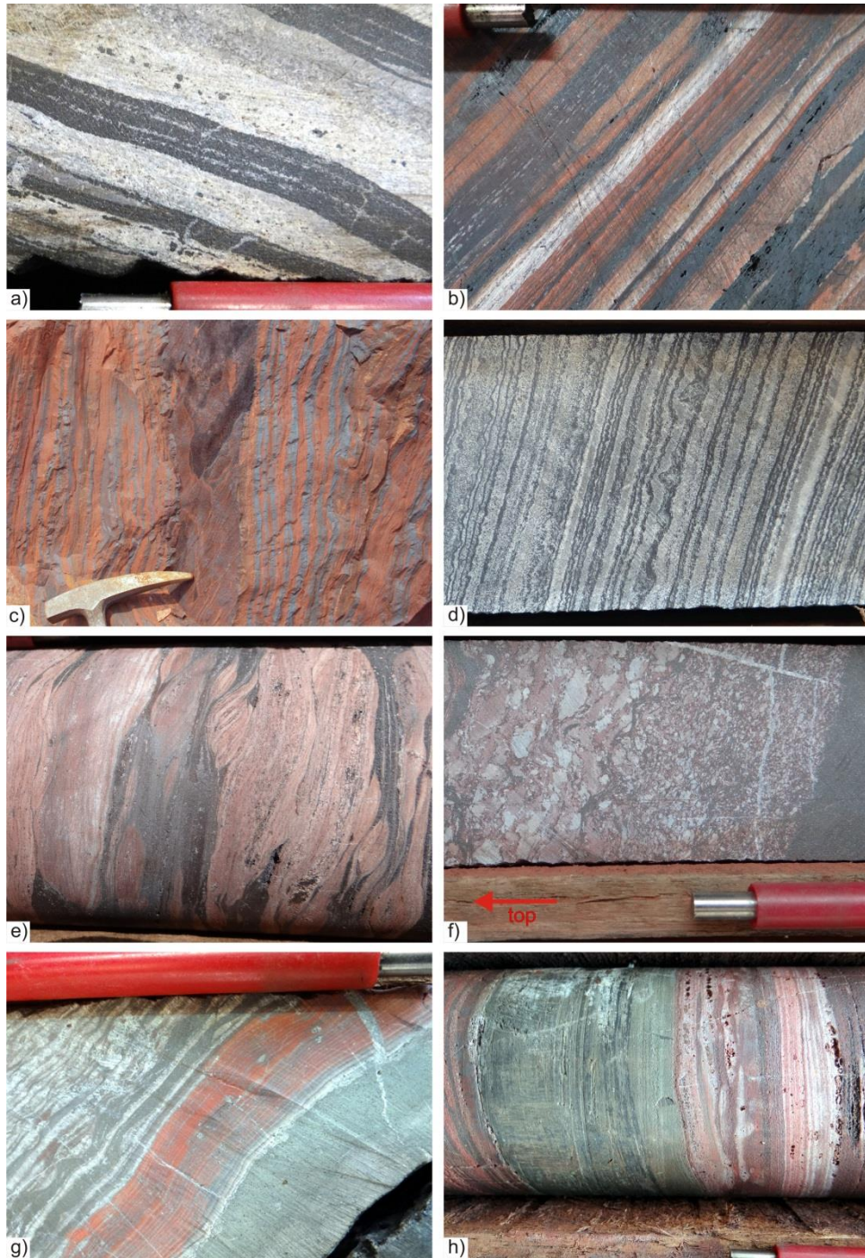
Fig. 3: Drill core (NQ=4.76 cm: a, d, g; HQ=6.35 cm: b, e, f, h) and outcrop (c) samples of Carajás IFs (in italic - drill core-sample id, depth, deposit, regional site): a) cherty-BIF (ALFA-FD01-453, 149.40-150.10 m, S11A, Serra Sul); b) mixed cherty-jasper BIF (N1-083-005; 186.40 – 186.70 m, N1, Serra Norte) c) jaspilite in the northern open-pit from N4E Mine (Serra Norte). Sedimentary textures: d) microbanding in cherty-BIF (GTCH-FD01-552, 388.65 – 388.70 m, S11B, Serra Sul); e) climbing ripples preserved as cross-poddings on pink jasper semi-destruct bands of jaspilite (N8-011-004, 120.30 – 121.20 m, N8 Serra Norte); f) ascending granocrescency in ressedimentated cherty-jasper band with metachert and jasper intraclasts possibly eroded still in pristine “gel-like” state (N1-288-013, 246.60 – 247.68 m, N1, Serra Norte). Lithologic associations: g) contact between basalt and jaspilite grading into cherty-jasper BIF, (ALFA-FD01-469, 353.05 -353.10 m, S11A, Serra Sul) and h) reduced pelitic layer interbedded with cherty-jasper BIF (N5W-576-009, 440.85 – 440.91, N5, Serra Norte).
