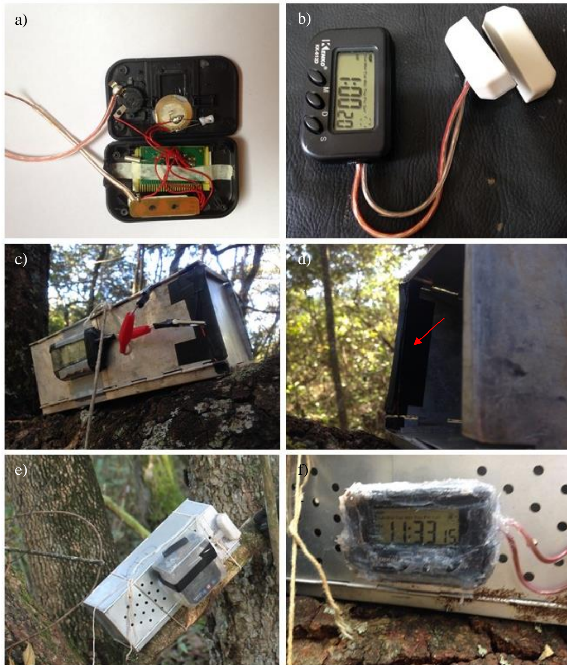
Figure 3. a) An opened digital clock to show the welded wires used to open the electric circuit. b) A clock with its electric circuit closed by magnets. c) Trap equipped with the first version of timer device protected with PVC. d) Red arrow indicates the bare wire that is on the inner side of the trap and touches the door when the trap is closed. e) Trap equipped with the second version of timer device inside a polystyrene box. f) Timer sealed with acetic silicone.
