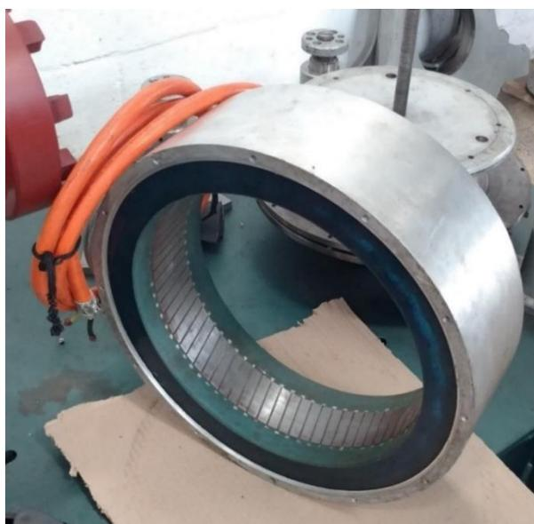
Figura 15 – Estator do PMSG.
