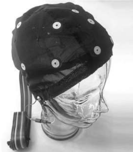
Figura 7. Touca para registro eletroencefalográfica Surgical Electro-CAP CS2005-M/L (Electro-Cap International, Inc. USA). Retirado de https://brain-trainer.com/wp-content/uploads/2013/10/electro-cap2.jpg .
