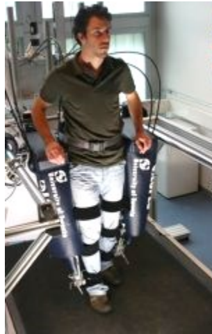
Figure 2.2 LOPES exoskeleton (year 2007) [12]
