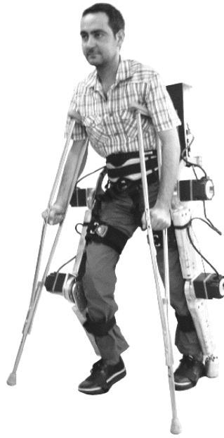
Figure 2.4 WSE exoskeleton (year 2014) [14]
