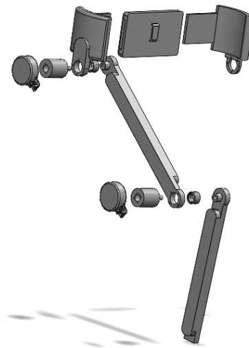
Figure 3.1 Solidworks Design of Exoskeleton
