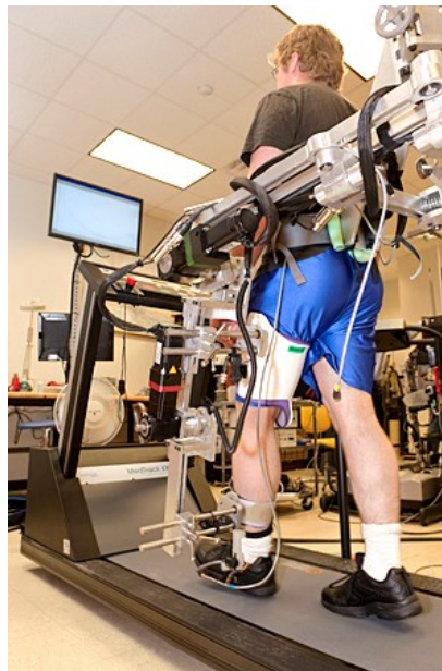
Figure 2.3 ALEX II exoskeleton (year 2011) [13]
