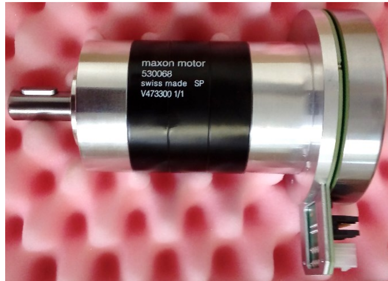
Figure 5.3 Maxon EC 90, brushless, 90 Watt motor with GP62 planetary gear
