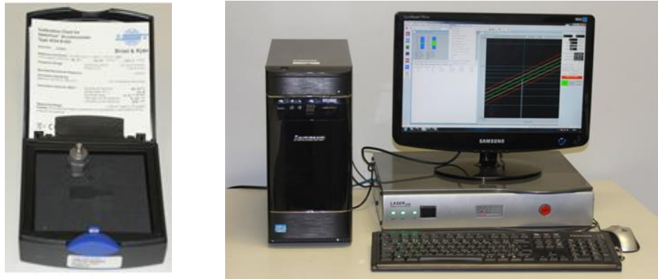
Figure 3.3: Type of accelerometer used (left) and the Laser usb LDS vibration controller and analysis system software (right)
