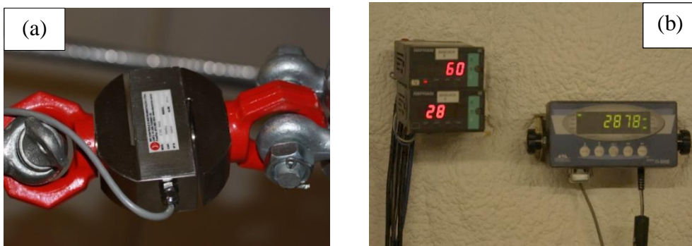
Figure 3.4: (a) The load cell used during the experiment; and (b) the indicator of the conductor stretching load
