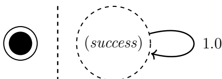
Figure 3.15: Transformation rule for an end node of an activity diagram
