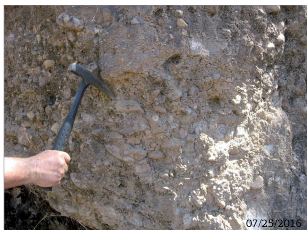
Figure 12. Detail of basal conglomerate of the basal Capacete Formation in the Canastrel digging. Note the lack of pebble sorting from top to base.
