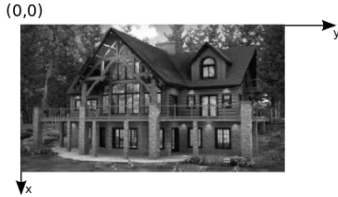
Figure 2.1: A digital image and the convention used for the pair of axes x and y .
