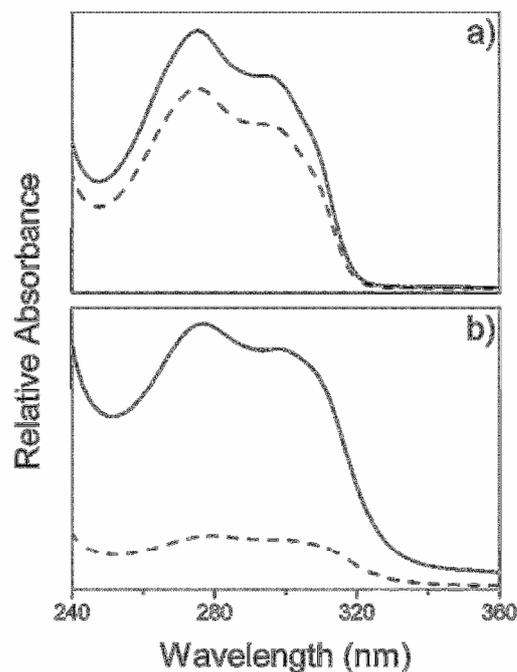
**Fig. 7.** UV-vis spectra of supernatant before (full lines) and after (dashed lines) interaction of mag@CS with tryptophan during drug loading process. In (a) Trp was loaded after magnetic composite synthesis and in (b) Trp was added during synthesis.
