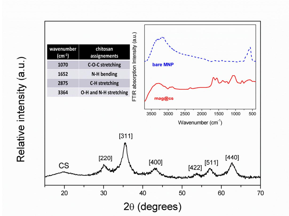
**Fig. 2.** X-ray diffraction pattern of mag@CS composite. Main diffraction peaks of the iron oxide (magnetite and/or maghemite) are identified by their indexes and reflection of chitosan is identified by CS. At the top right corner, the FTIR spectra of bare magnetic nanoparticles (dashed blue) and mag@CS sample (red). Inset table lists the main FTIR transitions for pure chitosan.
