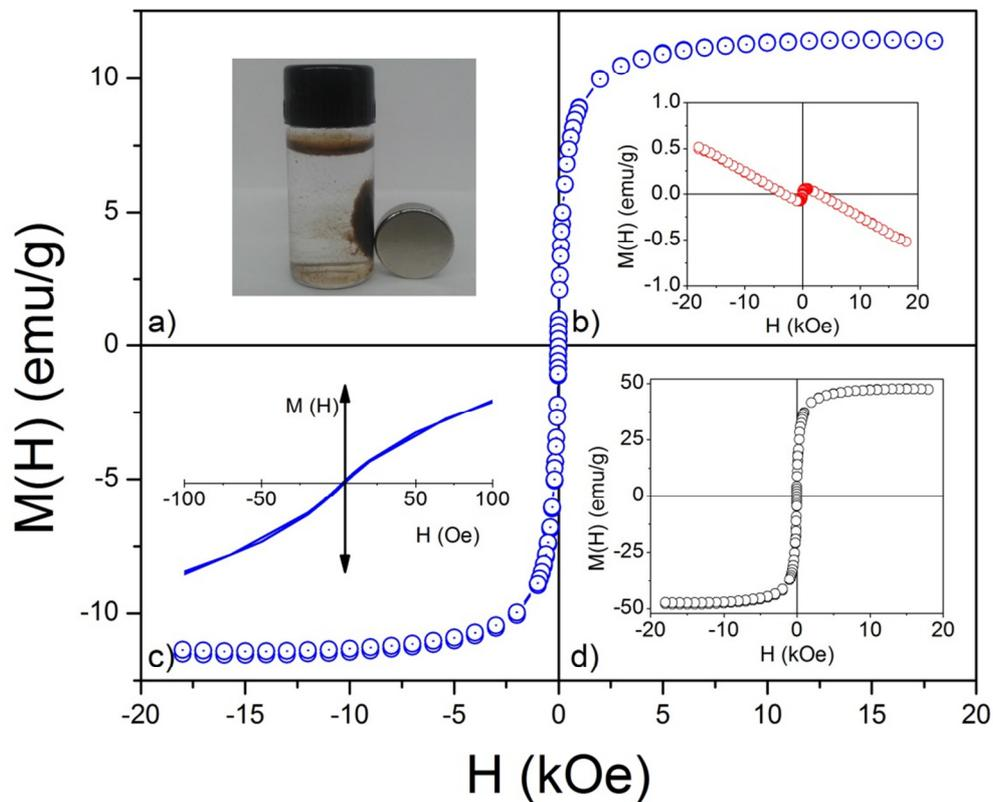
**Fig. 6.** Magnetization hysteresis loop at room temperature for sample mag@CS (blue circles). Picture of magnetic chitosan under action of a permanent magnet (a). Magnetization curve at room temperature of pure chitosan (b). Magnetization data of mag@CS at low field range (c) and normalized only by the iron oxide mass (d).
