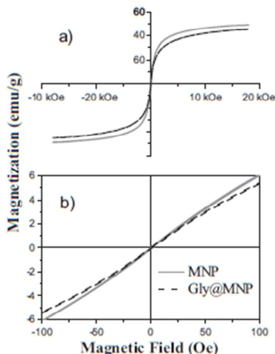
Fig. 3. (a) Magnetization curves of MNP and Gly@MNP samples. (b) Magnetization data at low field range.
