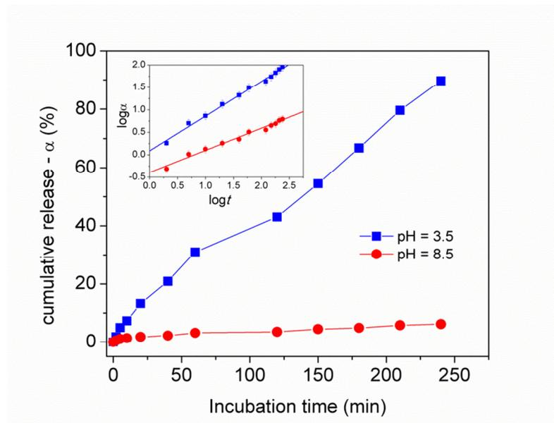
**Fig. 8.** Cumulative release of Trp as a function of time for mag@CS samples at different pHs. The inset is a log-log plot and full lines are the linear fit of data.
