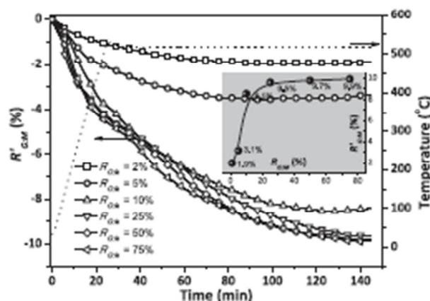
Fig. 6. TGA curves of weight loss versus time for functionalized NPs. Dashed curve represents the heating profile and the inset displays the amount of adsorbed glycine ( $R_{GM}$ ) as a function of glycine concentration used in functionalization ( $R_{GM}$ ).
