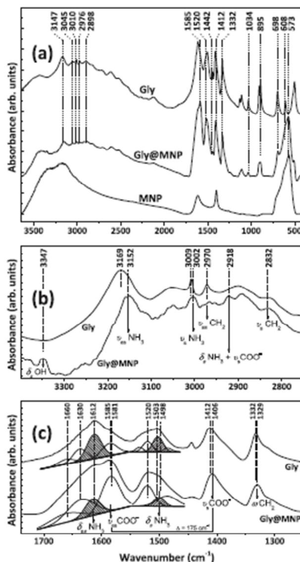
Fig. 7. (a) and (b) FTIR spectra of pure glycine, bare MNP and Gly@MNP and their correspondent assignments. (c) Gaussian band deconvolution procedure corresponding to the  $\delta(\text{NH}_3)$  and  $\nu(\text{COO}^-)$  envelope.
