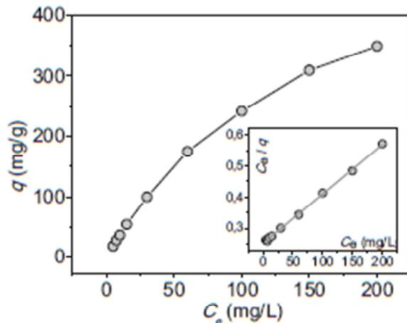
Fig. 11. Equilibrium isotherm for  $\text{Cu}^{2+}$  adsorption by glycine-modified maghemite nanoparticles at 25°C and pH=6.5. The inset shows the Langmuir adsorption isotherm fit of  $\text{Cu}^{2+}$  adsorption.
