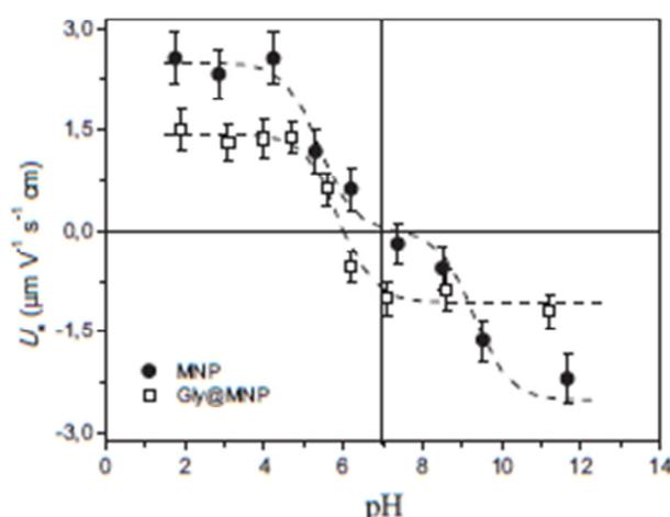
Fig. 5. Electrophoretic mobility ( $U_e$ ) of MNP (circles) and Gly@MNP (squares) slurries as a function of pH. Dashed lines are guides for the eyes using the models of surface charge that are described in the text.
