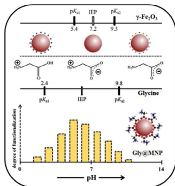
Fig. 4. Glycine adsorbate speciation and maghemite surface charge dependence on pH. The relative degrees of glycine adsorption (in arbitrary units) are plotted as a function of the pH at the bottom of figure for Gly@MNP.
