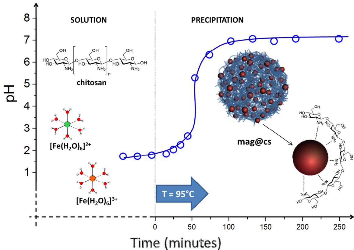
**Fig. 1.** Schema of synthesis of mag@CS nanocomposites. Circles are the variation of pH as a function of the time of reaction. Before 95 °C, iron complexes and chitosan coexists in solution. As temperature reaches 95 °C and time increases, chitosan polymerizes (blue thread ball) embedded with magnetic iron oxide nanoparticles (red spheres).
