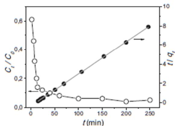
Fig. 10. Application of kinetic pseudo second-order linear model (gray line) to the experimental data (full circles). The open circles show the variation of copper concentration as a function of the time, using 7.5 mg of adsorbent and 50 mL of copper solution at  $\text{pH} = 6.5$  and  $25^\circ\text{C}$ .
