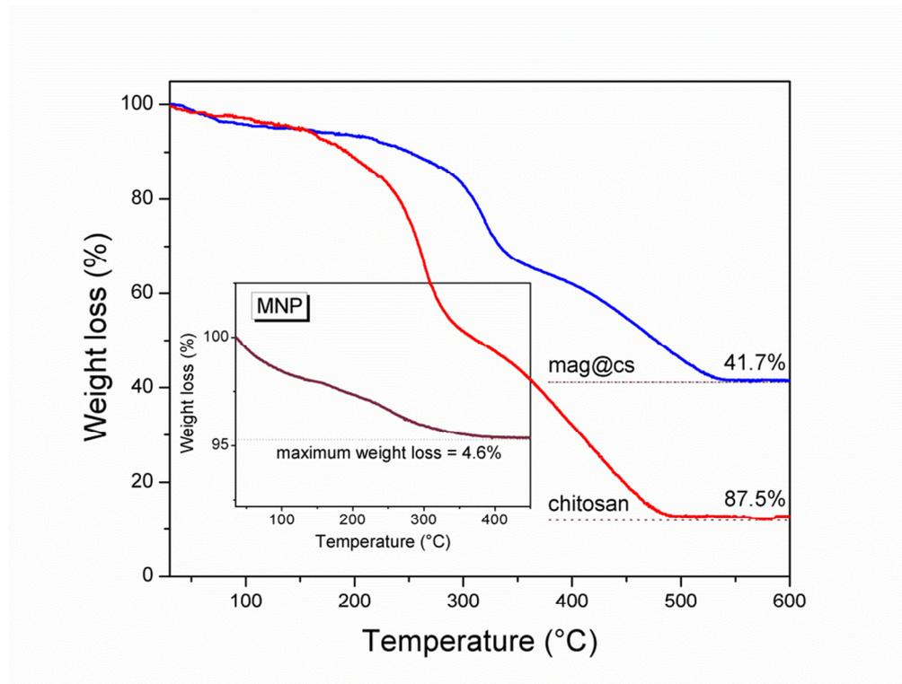
**Fig. 5.** Thermograms of mag@CS (blue) and pure chitosan (red) samples. The inset shows the weight loss observed in pure iron oxide nanoparticles.
