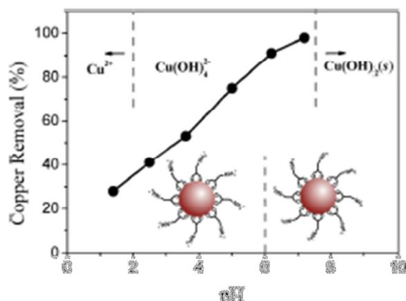
Fig. 8. Copper removal efficiency at different pH at 25 °C, using 7.5 mg of adsorbent 50 mL of 10 mg/L of  $\text{Cu}^{2+}$  and a contact time of 1 h.
