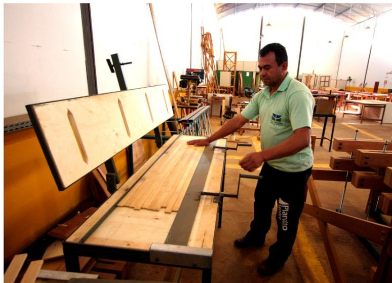
Figura 53: Prensa horizontal do CPAB/UnB.
