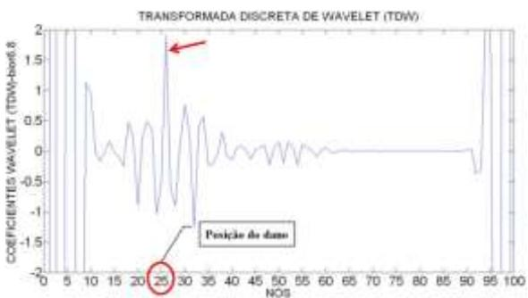
Figura 6.118- TDW viga V2E-2 usando bior6.8.
