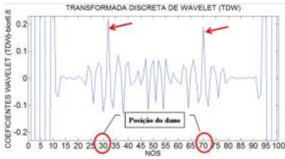
Figura 6.57- TDW viga V3E usando bior6.8.
