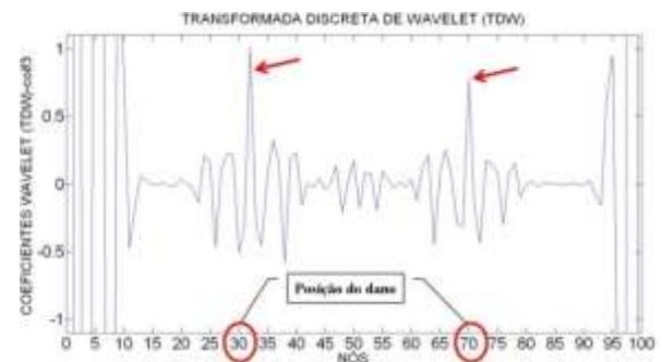
Figura 6.126- TDW viga V3E usando coif3.
