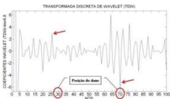
Figura 5.39- TDW viga V3E usando bior6.8.
