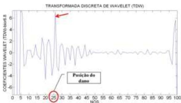
Figura 5.34-TDW viga V2E-2 usando bior6.8.
