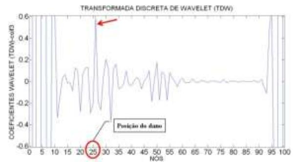
Figura 6.187- TDW viga V2E-2 usando coif3.
