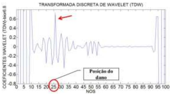
Figura 6.52- TDW viga V2E-2 usando bior6.8.
