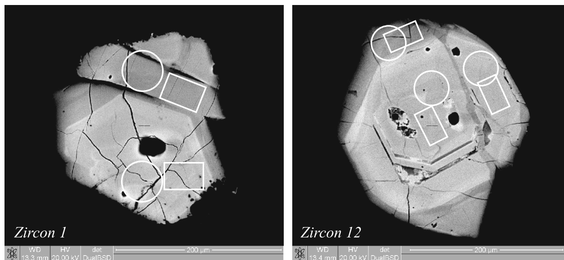
Fig. 3 – Backscattering images of studied zircons. White circles: Lu-Hf laser spot; white rectangle: U-Pb laser raster.
