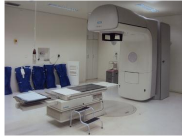
Fig.1 Primus linear accelerator, by Siemens, used by the University of Brasilia Hospital (HUB) in the radiotherapy sessions.
