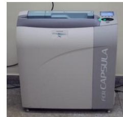
Fig.2 FCR digitizer by Fuji, used by the University of Brasilia Hospital (HUB) to acquire the digital radiographic image.
