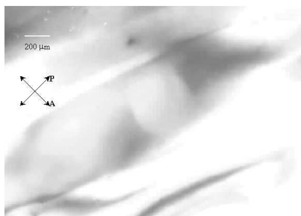
Figure 6. Sample of \text{CuFe}_2\text{O}_4 ionic ferronematic in microslide 400\ \mu\text{m} thick, observed in a polarized light microscope, in the presence of a magnetic field of 200 G (along the horizontal direction, in the plane of the figure). The texture was obtained 10 min after the application of the magnetic field.
