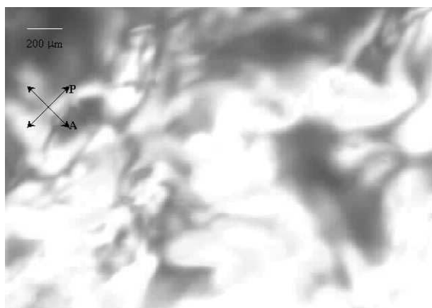
Figure 3. Sample of surfacted ferronematic in microslide 400\ \mu\text{m} thick, observed in a polarized light microscope, without the magnetic field.
