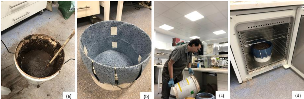
Figure 3.7. Preparation steps of the dense specimens using the “Air dried” technique.
