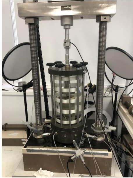
Figure 3.13. CSD test with shear wave velocity measurements.
