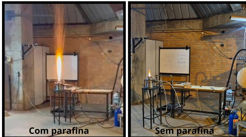
Figura 3.10 – Teste com end-burning / Teste sem end-burning.
